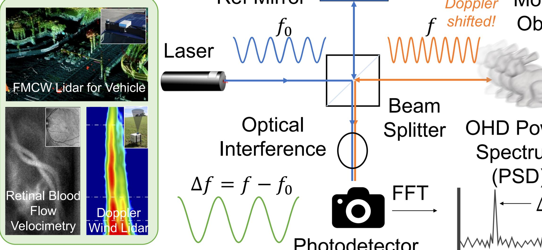
A broad range of imaging systems—including FMCW LiDAR, blood flow velocimetry, and wind Doppler lidar—can be understood within the unified framework of optical heterodyne detection (OHD). We developed a scalable Monte Carlo (MC) simulator that accurately models multipath effect in complex OHD scenarios. The key idea is to express the OHD measurement as a **path integral**, enabling the use of existing physically based light transport techniques.
